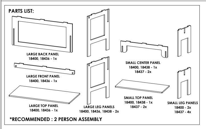
**STEP 1:** On an even flat surface stand the Large Leg Panels upright as shown below. While holding the Large Leg Panels upright, simultaneously slide the slots on the Large Back Panel into the slots in the Large Leg Panels. Slide the Large Back Panel down until the panels are fully engaged.
