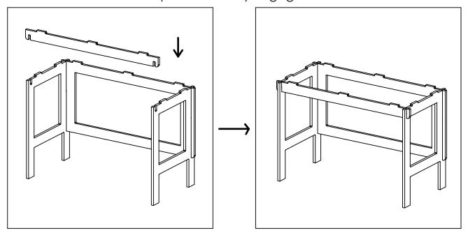
**STEP 3:** Align the bottom slots on the Large Top Panel with the top tabs on the Large Front Panel, Large Back Panel & Large Leg Panels. Place the Large Top Panel on top of the assembled unit until it fits securely.
