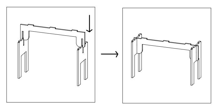
**STEP 3:** Align the bottom slots of the Small Top Panel with the top tabs on the Small Center Panel & Small Leg Panels. Place the Small Top Panel on top of the assembled unit until it fits securely.
